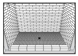
8. You are now ready to tile to the shower enclosure. Only Rapid Set thin-set/tile mortar or any type of modified thin-set/tile mortar should be used to lay tile on the pan. Adjust the height of the drain as necessary to accommodate the flooring covering.
