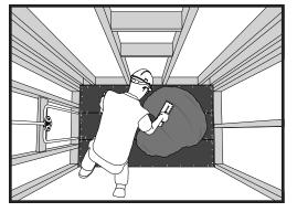
1. Frame out shower stall area to shower pan dimensions. The bore hole needs to be a minimum 6", but not more than 7" diameter opening\*. Ensure that the shower pan subfloor is level, and that the walls are level, plumb, and square. Place the square in corners to ensure they are square and straight. All walls and framing must be plumb prior to proceeding. The floor must be level within 3/8". Sweep up any debris from subfloor.
