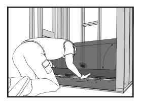
5. Place the pan on the thin-set bed and apply pressure or wiggle the pan a little to make sure the thin-set spreads out evenly under the pan so the pan makes proper contact with the modified thin-set. This process will ensure that the modified thin-set will fill in the footprint of the pan.
