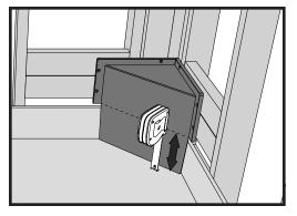
4. Once the shower pan is firmly butted up against the studded walls, measure the distance from the floor of the shower pan corner to the underside of the Redi Ledge. Use that measurement to make any height adjustments to the diagonal stud support so that the Redi Ledge sits on top of the support firmly.
