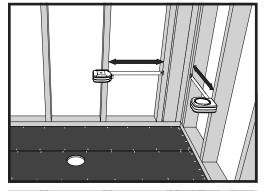
1. The corner of the shower stall where the Redi Ledge will be installed requires stud support. These Redi Ledge stud supports can be made from metal or wood, depending on the project requirements.
