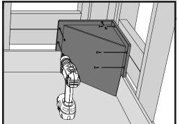
6. Level and mechanically fasten the Redi Ledge using one framing screw in each pre-drilled hole.
