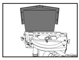
5. It may be necessary to trim the bottom of the Redi Ledge wall so that the Redi Ledge sits flush on the shower pan splash walls. This can be done with a table saw, circular saw, or a reciprocating saw.
