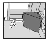
Neatly apply 100% waterproofing silicone to cover each screw head and to fill the gap between the Redi Ledge front, the floor of the shower pan, and the adjacent splash walls.
