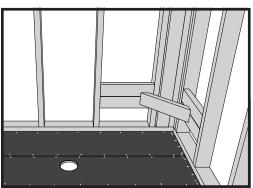
3. Now cut and mount a diagonal support bracket to allow for support to the underside of the Redi Ledge.
