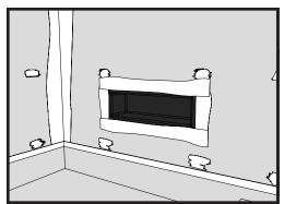
7. Then apply a liquid applied waterproofing membrane to all four ledge flanges and covering at least 1 inch of the adjacent tile backer board
