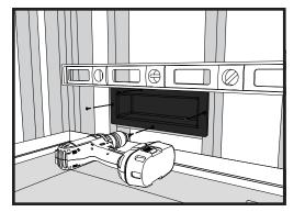
4. Level and mechanically fasten the Redi Niche using one framing screw in each pre-drilled.
