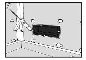
6. Neatly apply 100% waterproofing silicone to cover each screw head and to fill the gap between the niche flange and the adjacent shower board.
