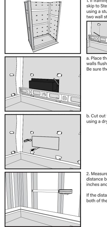
1. If framing Redi Ledge into an existing finished wall (if new construction, skip to Step 2), first locate and mark the center of adjacent framing studs using a stud finder or by tapping the wall. Draw a level line between the two wall studs.
