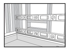
3. Measure and cut top and bottom horizontal support framing to a length which permits each to run between and to be fastened to both vertical studs. Level and mechanically fasten the top and bottom horizontal support brackets to both adjacent vertical studs so that the vertical dimension between the horizontal support framing matches the vertical dimension of the pre-drilled fastening holes on the Redi Ledge flange.
