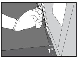
6. Offset the mortar base 1" from each outside edge of the pan with exception of the curb side. Mortar will protrude out from under the curb, run the finishing trowel along curb face to backfill any excess mortar. Mark a line on a shim denoting the distance calculated in Step 4. Use the
