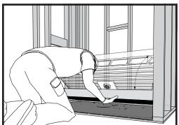
8. Place the pan in the mud base and firmly but gently shimmy the pan (applying pressure in drain location first) into the mud so that (i) the drain is fully supported by mud at the bore hole in the substrate, and (ii) the ribs are completely filled with the mud alternately applying hand pressure
