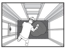
5. Spread your mortar base (should be a milk shake consistency), evenly across the subfloor at the thickness calculated in Step 4.
