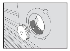
7. If there is access from the subfloor below and you followed Step 3a, then brush primer and PVC adhesive on the inside of the drain and outside of the cut drain pipe and quickly insert into drain connection, then be sure the drain pipe extends far enough below the subfloor so it can be connected to the waste water pipe following the installation.
