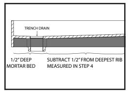
DO NOT PLACE THE MORTAR DIRECTLY ON A WOOD OR GYPCRETE SUBSTRATE. FIRST, WATERPROOF THE WOOD SUBSTRATE WITH A FLUID APPLIED WATERPROOFING MEMBRANE, OR NO. 15 OR NO. 30 ROOFING PAPER SO THE WOOD DOES NOT ABSORB THE WATER FROM THE MORTAR.
