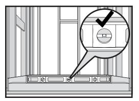
9. Using the level, ensure that the pan is level left to right, and front to back along the splash walls. Also make sure the pan is level left to right along the curb.
