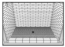
11. Adjust the height of the drain as necessary to accommodate the floor covering. Set your tile using a white modified thin-set/tile mortar and a notched trowel as specified by the thin-set/tile mortar manufacturer based on your tile size. Tile Redi recommends the modified thin-set/tile mortar products found in table below.
